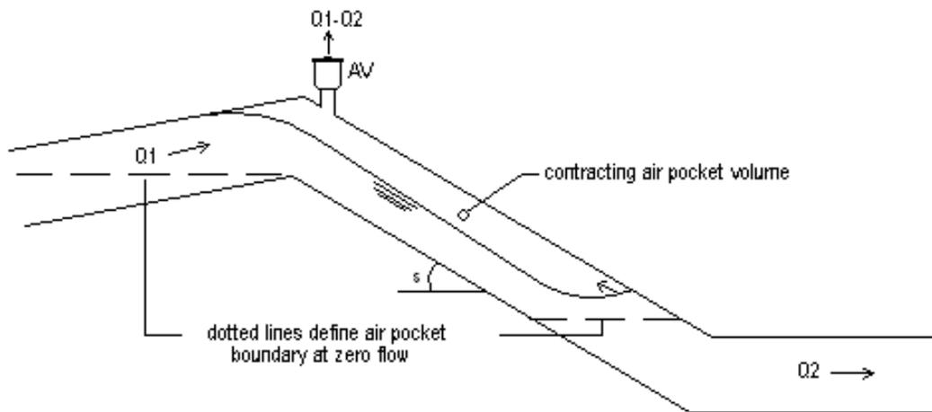
**Fig 3 Air-release valve schematic**
