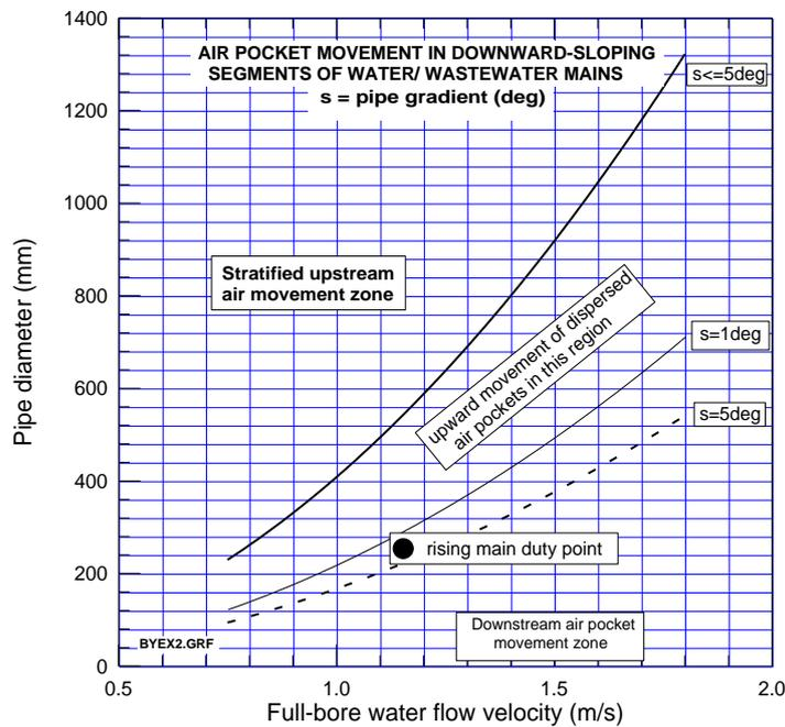
**Fig 7** Example 2 rising main air pocket movement prediction
