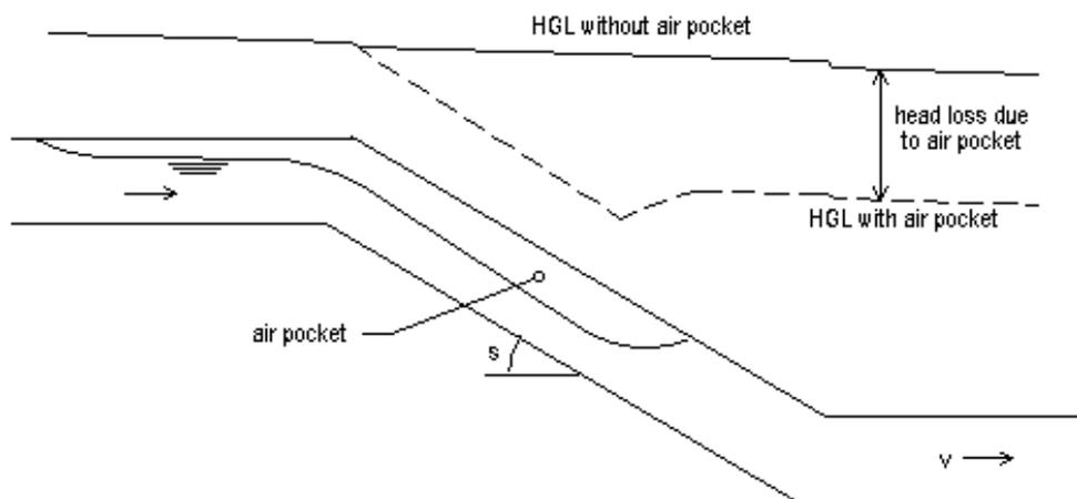
Fig 1 Pipeline trapped air pocket schematic
