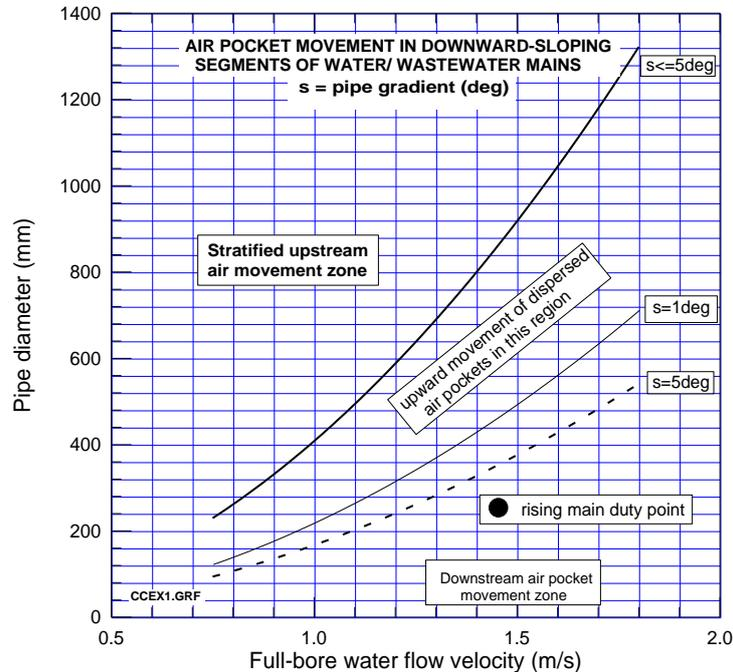
**Fig 5 Example 1 rising main air pocket movement prediction**
